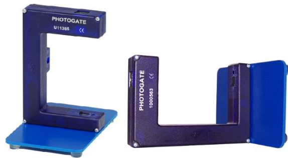
Fig. 3: With holding plate e.g. in experiment with torsion apparatus or reversible pendulum
