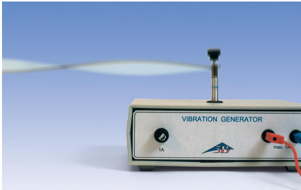
Fig 1 Experimentel set-up with the rubber band
