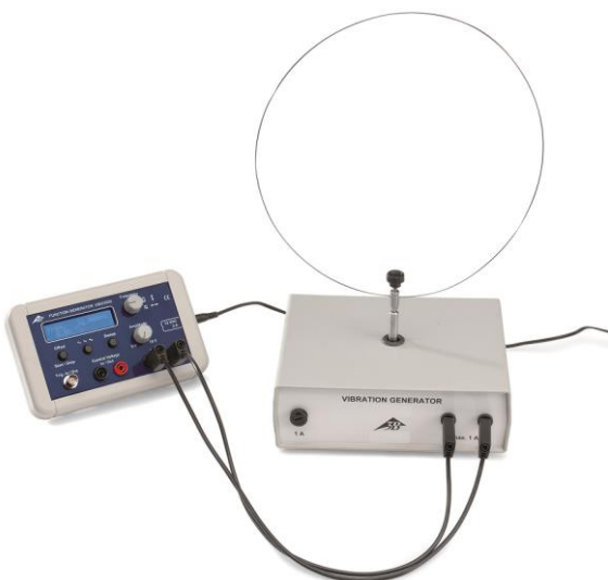
Fig. 3 Experimentel set-up with the resonance wire
