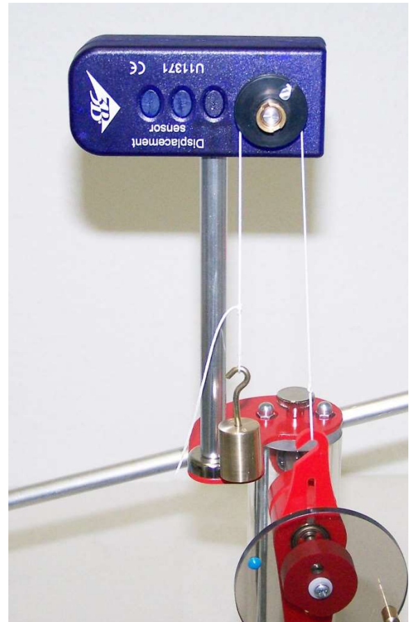
Fig. 5: Attaching the thread to the hook on the connector rod
