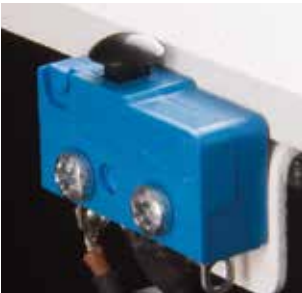
Figure 4: Safety limit switch 1
