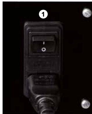
Figure 29: Main switch (1) on the back of the simulator
