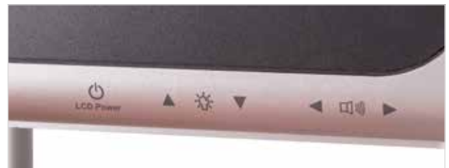
Figure 13: Controls on the monitor
